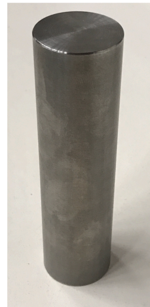
Fig. 14. Titanium cylindrical object, ( L_{co} = 130 , • D_{co} = 35 mm), \rho_p = 4,464 kg/m 3 .
